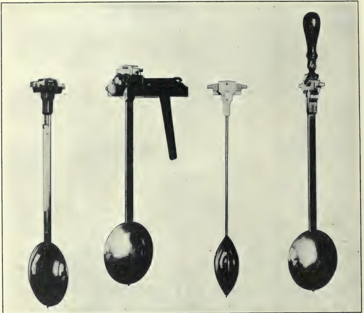
FIG. 2.—MENDENHALL HALF-SECOND PENDULUMS AS ORIGINALLY CONSTRUCTED WITH KNIFE-EDGE ATTACHED TO HEAD OF PENDULUM AND DIVIDED INTO TWO PARTS.
